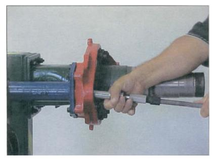
Insert collet into s-cam bracket hold collet and turn the shaft to expand it larger than the bushing
