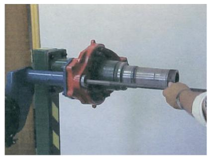
Insert slide hammer shaft into the driver and out the backside of the s-cam bracket
