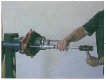
Hold collet against the back bushing. drive bushing and seal out the backside
