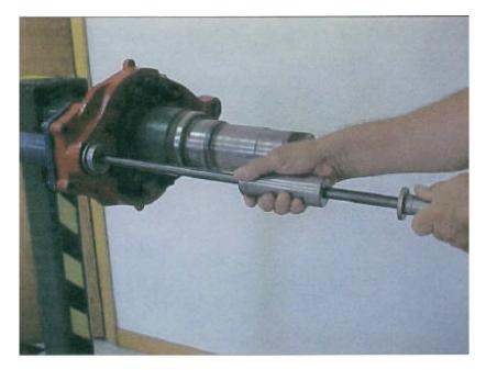
Pull handle against the inside bushing. Using slide hammer, pull out inner bushing and seal.
