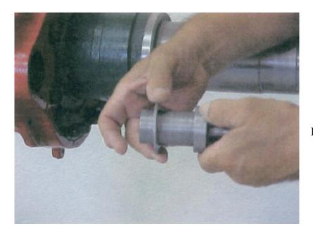
Remove driver and install large washer
