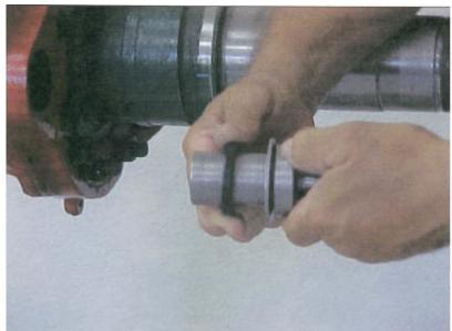
Install s-cam seal (lip facing slack adjuster) against the washer. Drive the seal into the spider.
