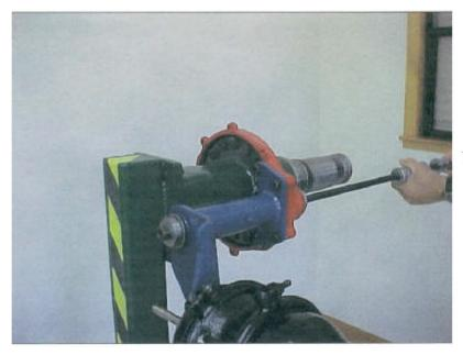
Phone: 916-635-8181 Fax: 916-635-8183 WWW.STROPPINI.COM Use slide hammer to pull the seal into the s-cam bracket in the same manner as the bushing
