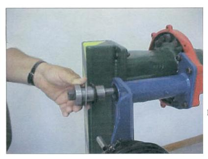
Remove the nut and driver, install the large washer and the seal (lip facing the slack adjuster)
