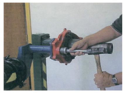
Insert short driver handle. Drive bushing into spider until it stops
