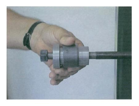
Install new bushing onto the second bushing driver. Secure the nut
