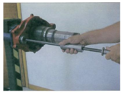
Use the slide hammer to pull the bushing into the s-cam bracket until it stops.
